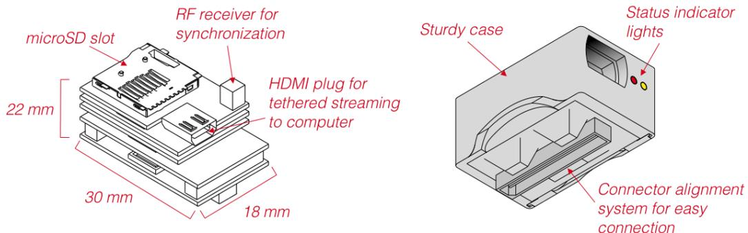
Figure 1- 128-Channel data logging headstage (HH128) diagram
