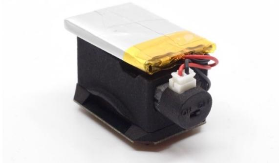
*Figure 4- HH128 connected to 400mAH battery for untethered data logging*
