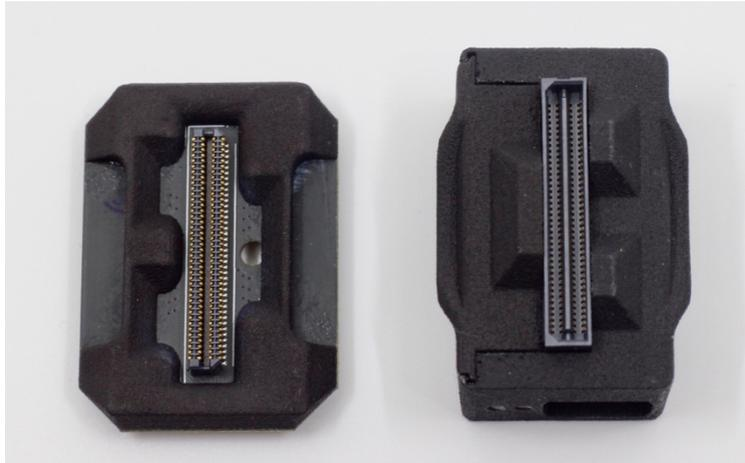
*Figure 2- Hardware channel mapping of the Lynx connector- a feature that offers a simple, robust system for headstage connection.*
