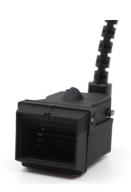
For untethered recordings, power (3.7 – 5V) must be supplied through the HDMI connector on the system using the SpikeGadgets power adaptor. Typically, a 3.7V rechargeable lithium battery is used. Also, a microSD card that has been formatted using the SpikeGadgets Logger Dock must be inserted into the SD card slot of the headstage. Once power is supplied, a set of possible LED indication patterns on the headstage signify system state:
