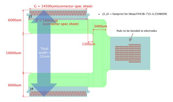
Figure 2- Flexible PCB routing the channels between the probe and the 128-channel modules
